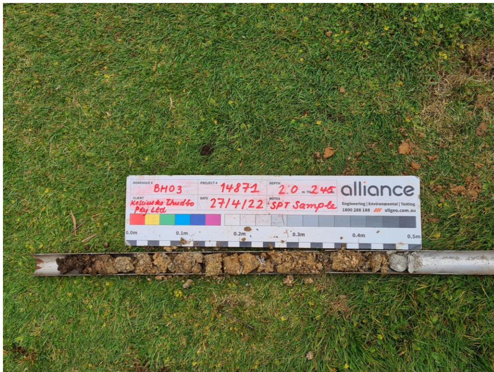
Photo 6 - SPT Split Spoon Samples at BH0, 2m-2.45m (N=32)
