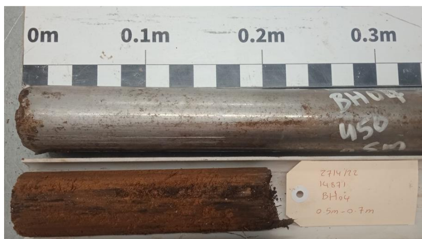
Photo 8 - U50 at Borehole BH04, 0.5m-0.7m
